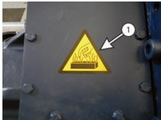
Figure 16-25: Gearbox inspection plate
