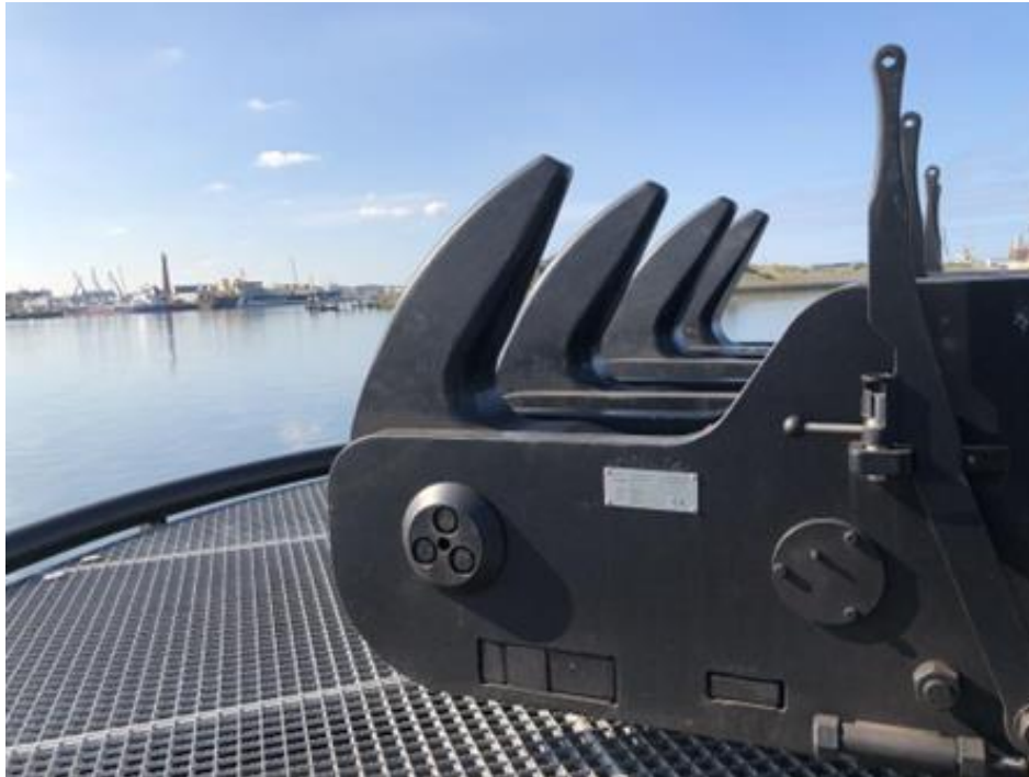
Figure 6-1 Example Quick release hook (Source: Straatman)
